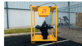
Duplex Strainer Skid
