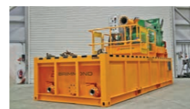
Modular Solids Recovery System
