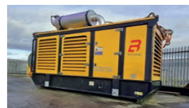
500kW Diesel HPU Safe Area
