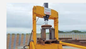
Hydraulic Press – Tests up to 1000Te
